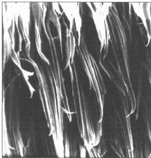
FIGURE 10 Fibrillar structure of split Nylon 6 fiber.
